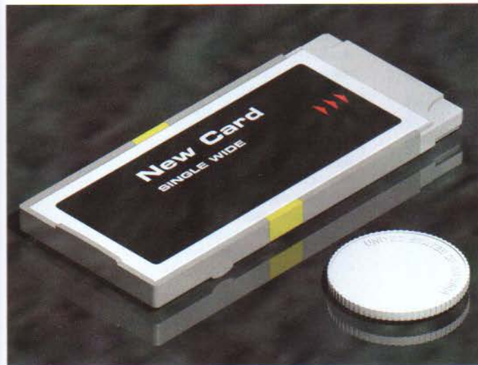
One result of PCI Express is a new form factor for add-ins. Currently labelled NEWCARD, these hot-swappable sealed units will bring the ease of use of USB to complex systems
